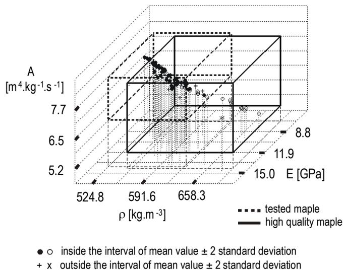
Fig. 2 The density  $\rho$ , the acoustic constant  $A$  and the Young's modulus  $E$  of individual test specimens of the high-quality maple and the tested maple.
