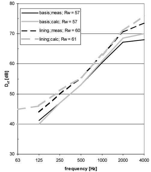
Figure 6: Measured and calculated sound level difference between living rooms with a  $465 \text{ kg/m}^2$  party wall, without (basic) and with (lining) an additional lining ( $\Delta R_w = 16 \text{ dB}$ ).
