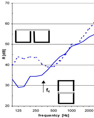
Figure 3: Sound reduction index for direct (—) and flanking (---) transmission; from [21].
