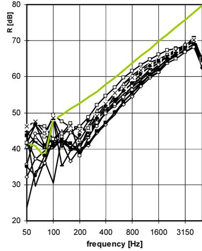
Figure 4: Measured sound reduction index of a 440 kg/m<sup>2</sup> wall in various laboratories with mass-law curve for comparison; from [22].
