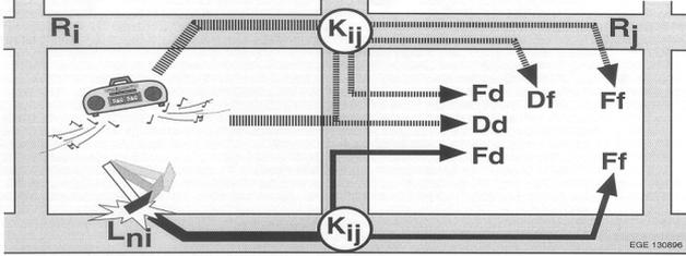
Figure 2: Illustration of direct (Dd) and flanking (Ff, Fd, Df) transmission path for airborne and impact sound transmission.
