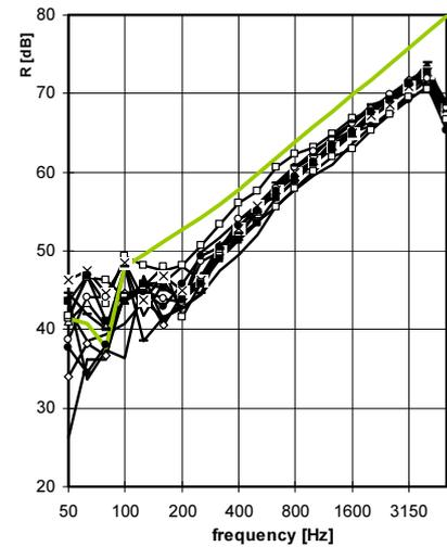
Figure 5: Results as in figure 4 after standardization to a typical laboratory structural reverberation time for resonant transmission; [23].
