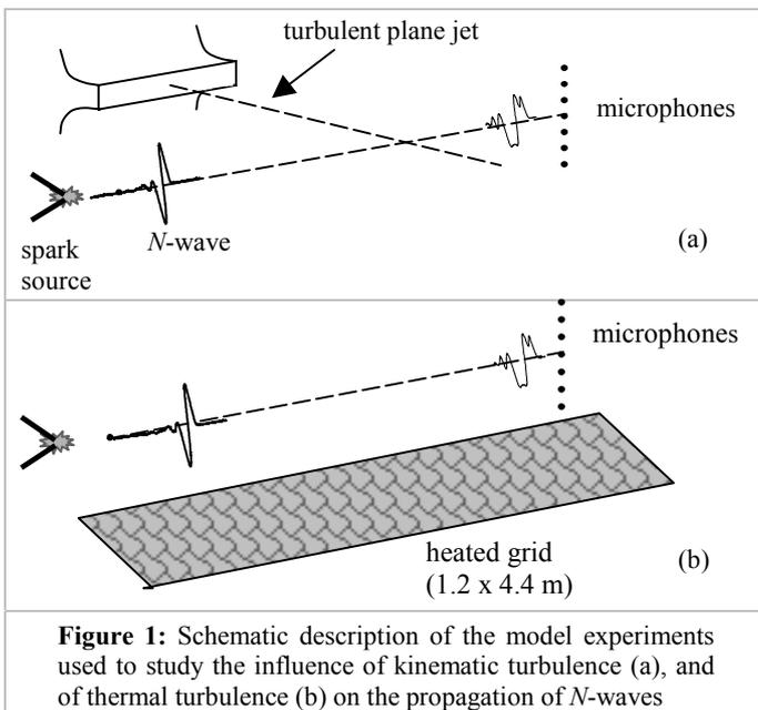
**Figure 1:** Schematic description of the model experiments used to study the influence of kinematic turbulence (a), and of thermal turbulence (b) on the propagation of  $N$ -waves
