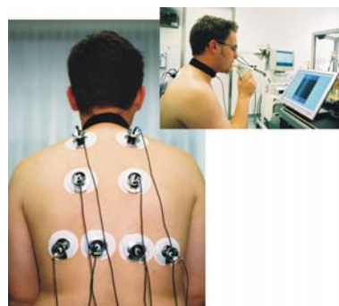
Figure 3: Eight sensors were mounted on the thorax and one on the trachea; the person had to breathe into an spirometer
