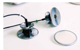
Figure 1: Newly developed sensors for picking up respiratory sounds; miniature microphones are integrated in
