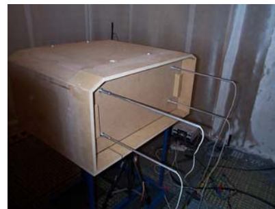
Figure 2: model of the engine compartment and the slots with the measurement microphones
