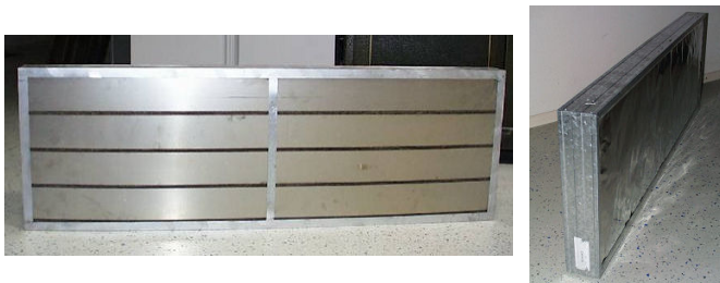
Figure 1: Silencer splitters as Slot Absorbers with horizontally arranged slots (left) and as Panel Resonators (right).
