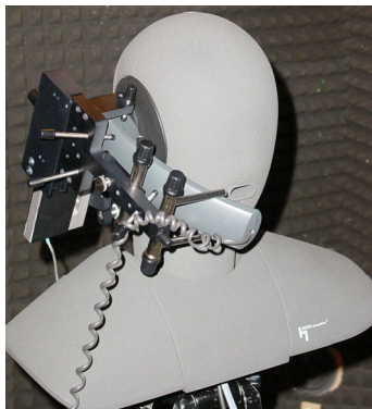
Fig. 1: HATS HMS II.3 with mounted ISDN phone)
