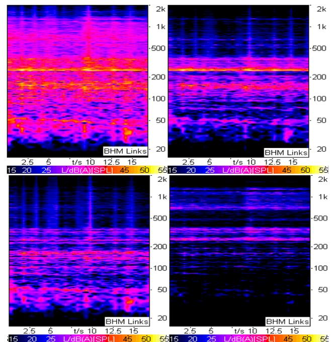
Figure 2: Road noise spectrograms: interior noise recording (top left), front axle structure-borne contribution (top right), rear axle structure-borne contribution (bottom left), airborne sound of all wheels (bottom right)
