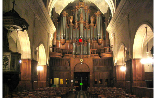
Figure 2: The Grand Organ of the Church St. Elisabeth du Temple, Paris, France. Loudspeaker (red) and balloon (green) source positions indicated.
