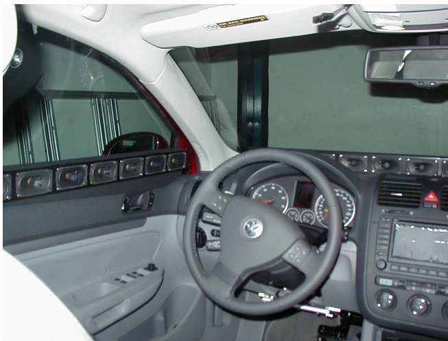
Figure 2: Full vehicle driving simulator with WFS set-up
