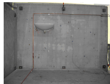
Figure 1: Pipe system with three segments mounted on three-plate reception rig.
