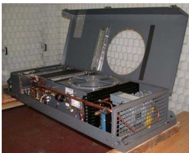
Fig. 1: General view of the HVAC unit with open lid (the compressor can be seen behind the grille in the foreground).
