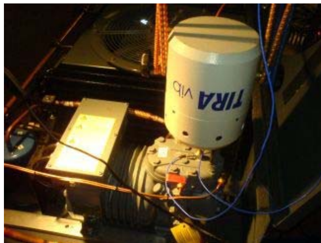
Fig. 2: The electrodynamic shaker attached to the top of the compressor (with force sensor and accelerometer).
