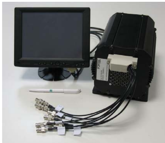
Fig. 4: Embedded PC system (PC/104 [3]) used for control.
