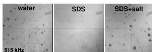
**Abbildung 1:** Cavitation at 515 kHz (frame width  $\approx 1$  cm, exposure time 0.8 ms). SDS: 1 mM, Salt: 0.1 M  $NaClO_4$ .
