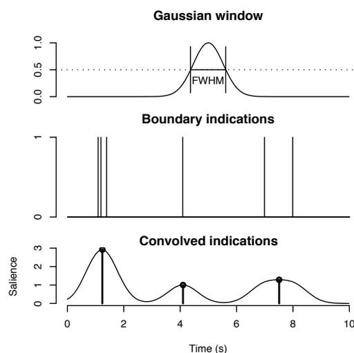
**Figure 1:** Visual representation of the Gaussian smoothing. The top row shows the Gaussian function with the full width at half maximum of 1.25 s, the second row some examples of indicated boundaries, and the third row shows the indicated boundaries convolved with the Gaussian function resulting in the smoothed boundary profile with the relative maxima, which are taken as the time points of a boundary.
