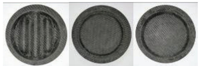
Figure 4: Composite simplified gear box lids (SGLids)
