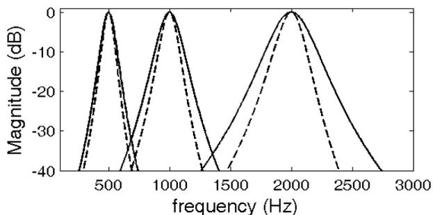
Fig. 4: Power spectrum of proposed gamma-chirp BP filters (dashed lines) and “standard” gammatone filters (solid lines).
