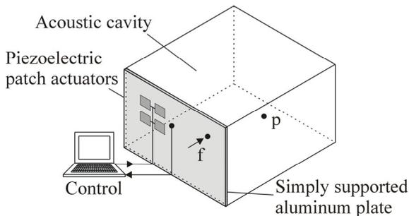
Figure 1: Smart plate coupled with an acoustic cavity
