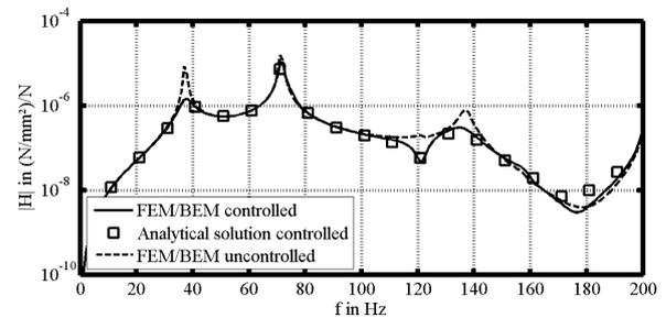
Figure 3: Comparison of the frequency responses with and without control
