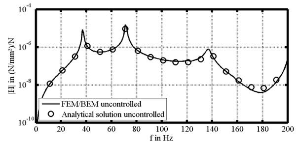
Figure 2: Comparison of the numerical and analytical frequency responses without control
