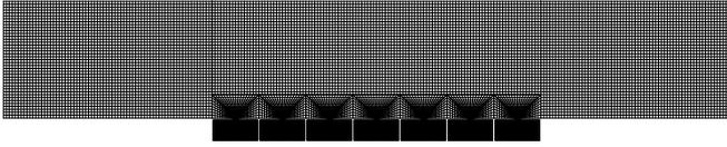
**Figure 1:** Part of the computational domain for the geometrically detailed hard-wall test case. The cell dimension inside the cavities is a tenth of the one in the duct section. The complex geometry and the requirements of the spatial-discretisation approach imply an acoustically over-resolved mesh (only plane-wave propagating patterns are introduced as acoustic excitation) and a very small time step.
