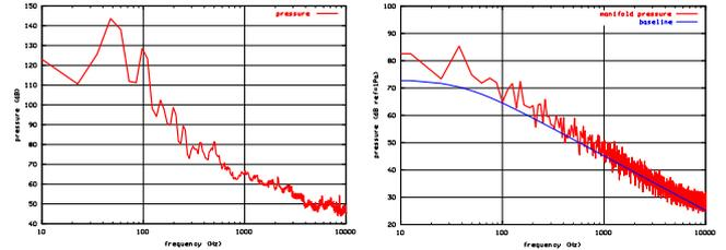
Figure 9: Measured (left) and simulated (right) exhaust power spectrum.
