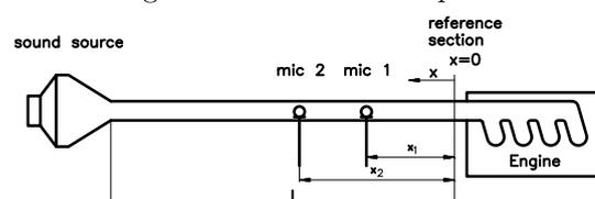
**Figure 4:** Measurement of the exhaust acoustical impedance. exhaust has been measured using the ISO-10534-2 two mi-
