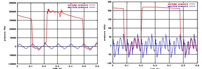
Figure 8: Measured (left) and simulated (right) pressure in cylinder and exhaust manifold.
