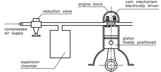
**Figure 2:** Scheme of the cold engine setup.
