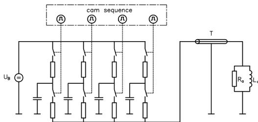
Figure 7: Circuit for cold engine setup in time domain.
