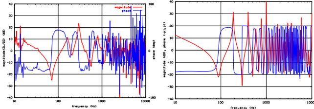
Figure 6: Measured (left) and simulated (right) exhaust impedance (0 dB= characteristic duct impedance).
