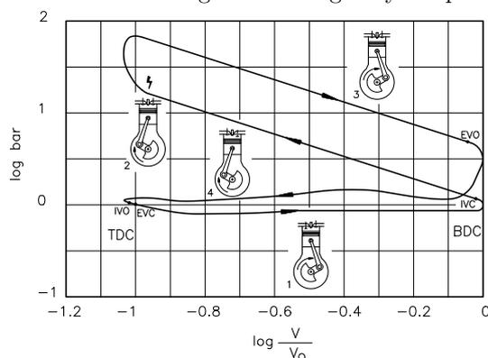
**Figure 1:** Indicator diagram of an internal combustion engine. the cycle repeats. The blowdown phase is responsible for the exhaust noise. The piston displacement during the blowdown phase is rather small, such that the exhaust noise can be considered as a discharge of a constant volume. The test rig, presented schematically in figure 2, is based on discharging constant volumes. It consists of a
