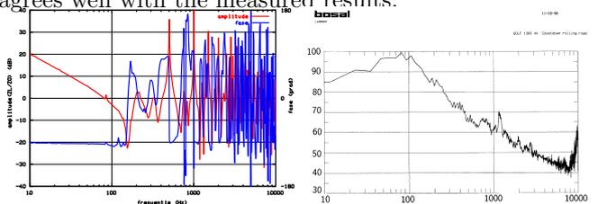
Figure 10: Exhaust impedance (left) and exhaust power spectrum (right) of an operational engine.
