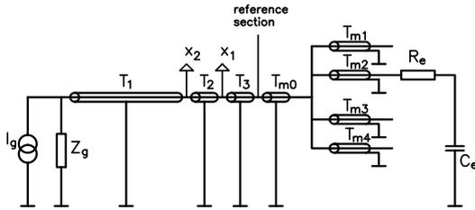
Figure 5: Electrical circuit for an engine in frequency domain.
