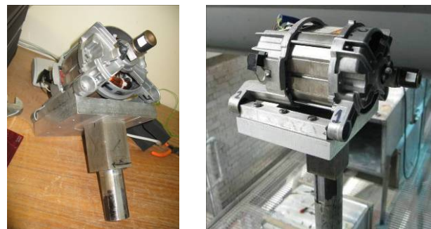
Figure 2: Electric motor used to represent a micro wind turbine for lab tests. Left: uncoupled, right: pole mounted.
