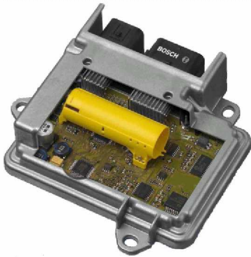
Figure 3: Electronic control unit with non-homogeneous contact pressure distribution in joints.
