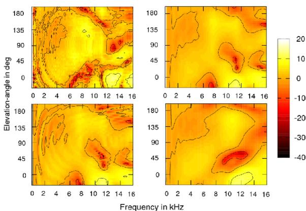
**Figure 2:** HRTFs for the median plane. TOP LEFT: Measured data. TOP RIGHT: Calculated data using high-quality mesh without torso. BOTTOM LEFT: Calculated data using high-quality mesh with torso. BOTTOM RIGHT: Calculated data using low-quality mesh without torso. [10]
