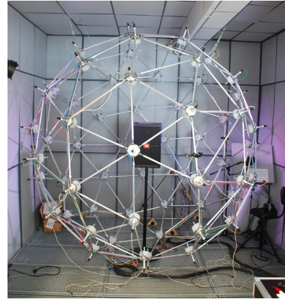
Figure 1: Surrounding 64-channel spherical microphone array in the semi-anechoic chamber at the IEM.
