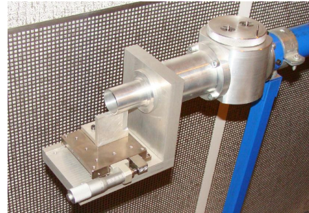
Figure 2: Photo of the damping device.
