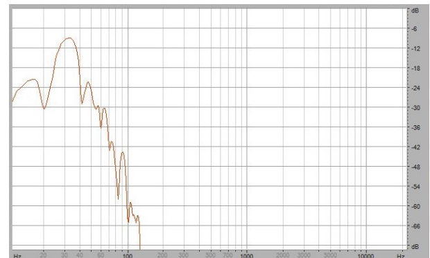
Figure 3b): Spectrum of generated sub-harmonic signal (calculated by a 16384-point FFT and a Blackman-Harris window function)
