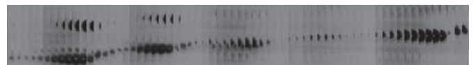
Figure 1: Pseudo-streak image of bubbles in water below a sonotrode tip driven at 20 kHz (subsequent vertical frames recorded at 250 kfps corresponding to 12.5 frames per driving period; exposure time 1 \mu s, image height 0.5 mm.) Note the lower bubble which is oscillating strongly in volume and jumping upwards during the collapse phase.
