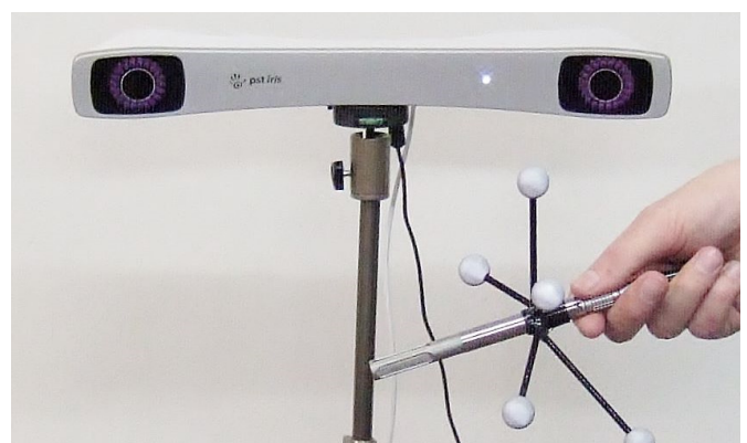
Figure 1: Stereo camera system tracking the movement of spherical reflectors attached to a 3D intensity probe.
