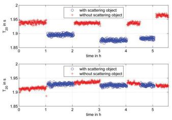
**Figure 2:** Reverberation time T20 over the measurement period of .5 hours. The measurements with scattering object present are marked with (blue) circles and without wit (red) crosses.
