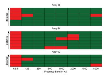
**Figure 3:** Results for the ANOVA analysis for every microphone position and frequency band. Significant effects of the presence of the scattering object are marked in green and insignificant in red.
