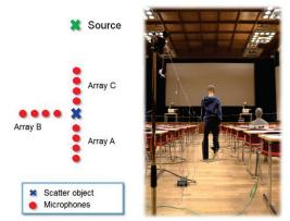
Figure 1: Overview of the measuring arrangement on the left side and photo of the measurement on the right.
