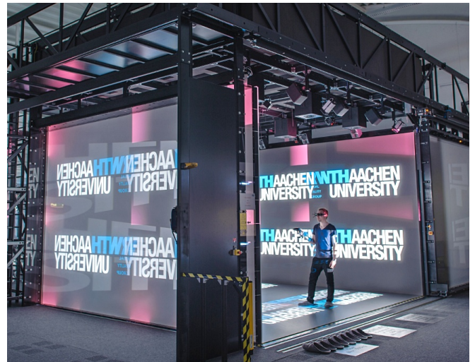
Figure 1: The aixCave in Aachen. Five sides are glass walls (with closed door) and the ceiling is acoustically treated. A loudspeaker system is mounted under the ceiling.
