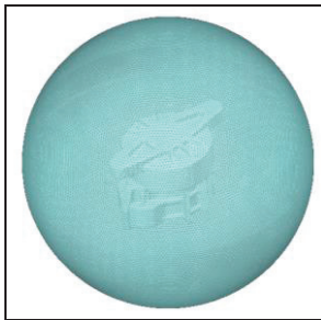
Figure 7: Finite element mesh for the Actran analysis: fluid volume mesh and outer boundary condition (Infinite Elements).
