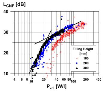
Fig. 9: Measured  $L_{CNF}$ -values drawn against the volumerelated effective power density (see text), obtained with a device with the half of the S900 bottom area (see text) at three different filling heights.
