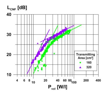
Fig. 10: Measured  $L_{CNF}$ -values drawn against the volumerelated effective power density (see text) as obtained at filling height 200 mm for the two different sound radiating areas of devices S900 and half of S900 (see text).
