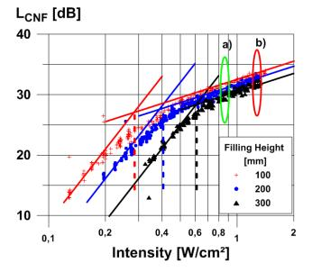
Fig. 6: Measured cavitation noise level L<sub>CNF</sub> drawn against measured values of the assigned intensities as obtained for the device S900 (see text) at three different filling heights. (Vertical lines mark the break points at thresholds of inertial cavitation. Circles a) and b) mark the region above the thresholds investigated in Fig. 7 in more detail.)
