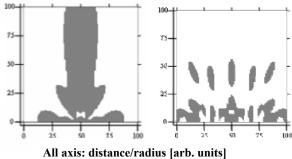
Fig. 3: Area with a sound pressure above the threshold of 100 kPa for a 3x3 array with small distance (left) and a high distance between the transducers (right)
