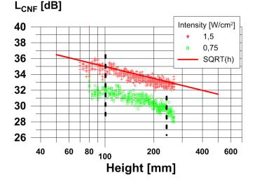
Fig. 7: Measured  $L_{CNF}$ -values drawn against filling height as obtained at two intensities for the device S900 (see text).
