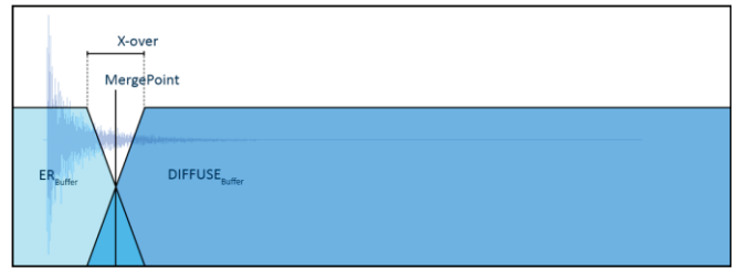
Figure 4: Linear merging of early and late reverb buffers.
