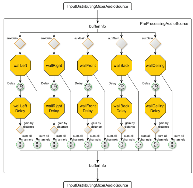
Figure 5: Audio signal flow chart to preprocess the incoming audio data and prepare for convolution.
