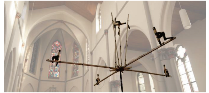
Figure 1: Microphone rig in the St. Dionysius church in Cologne with microphones each pointing to a different wall.
