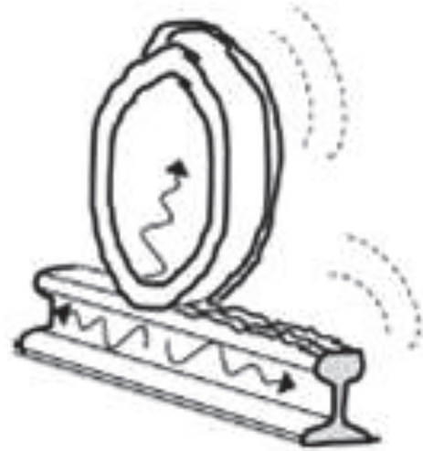
Figure 1: A railway wheel rolling on a railway rail with surface roughnesses. The rail/wheel contact force excites rail and wheel into vibrations which radiate away in the air as noise.
