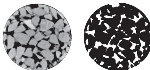
**Figure 5:** One horizontal slice from a CT-scan of a porous asphalt concrete bore cores (PAC 11/16); **left:** grayscale image (black = air, dark/light gray = bitumen/stone); **right:** binary image of the same slice, with white indicating the air voids
