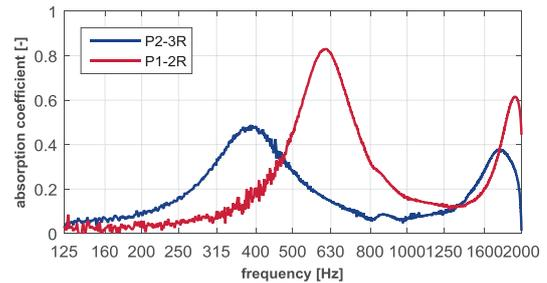
**Figure 9:** Sound absorption measurement results for bore cores P1-2R and P2-3R
