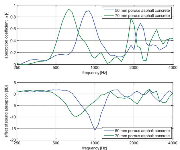
**Figure 2 top:** sound absorption spectrum measured in-situ on porous asphalt concrete (50 mm single layer, 70 mm double layer); **bottom:** reduction of the horn amplification measured on these surfaces
