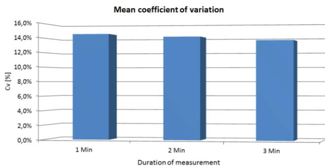
**Figure 1:** Mean coefficient of variation of 35 acoustical parameters of 13 repeated measurements in dependence of measurement duration
