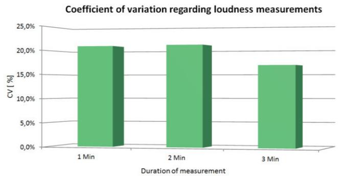
**Figure 2:** Coefficient of variations of loudness measurement results of 13 repeated measurements in dependence of measurement duration
