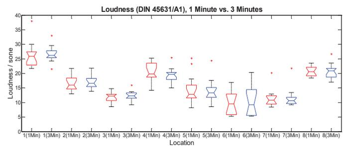
**Figure 3:** Box-whisker plot: Loudness measurement results of 13 repeated measurements per location. Red: Loudness results of measurements with a duration of 1 minute; blue: Loudness results of measurements with a duration of 3 minutes
