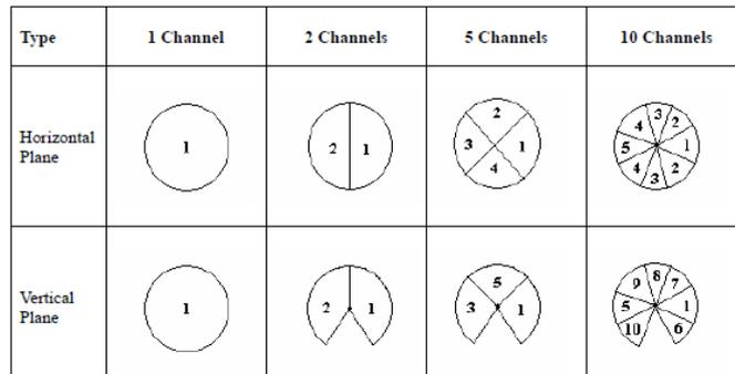
**Figure 1:** partial sources used for multi-channel source directivity auralizations (from [2]).
