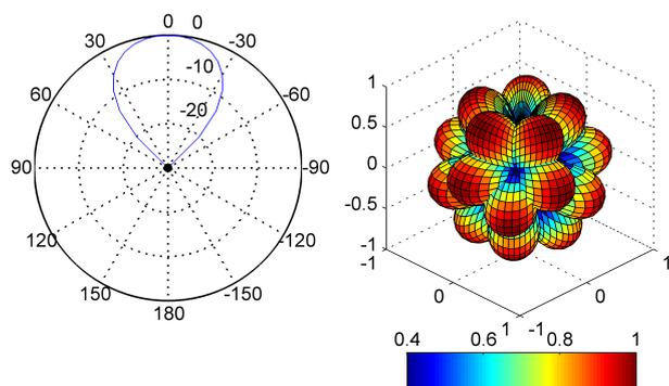
**Figure 2:** (left): 2D polar plot of a single beam (dB scale), and (right): superposition of the 20 3D beam patterns (linear scale) to show orientations.
