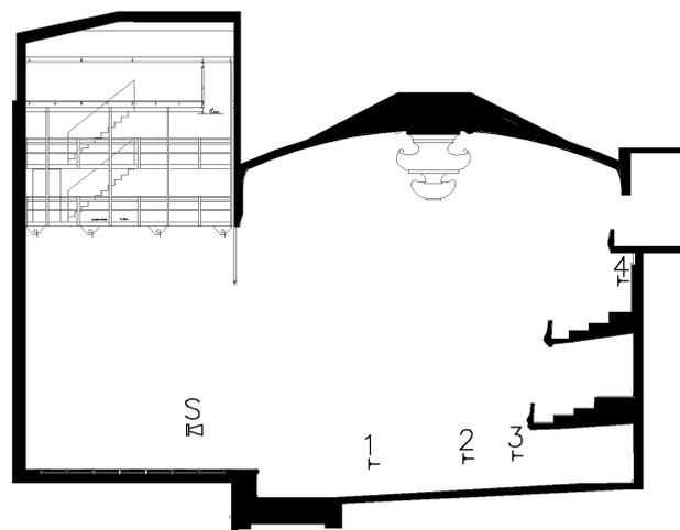
**Figure 3:** Section of the Théâtre de l'Athénée depicting the source position on stage and the 4 receiver positions (1, 2, 3 first floor, and 4: third floor)
