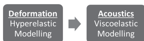
Figure 1: Analyses of a seal system as a two-step procedure
