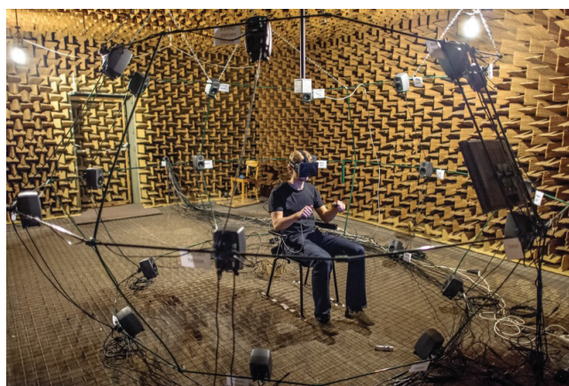
Figure 1: Example for periphonical loudspeaker array
