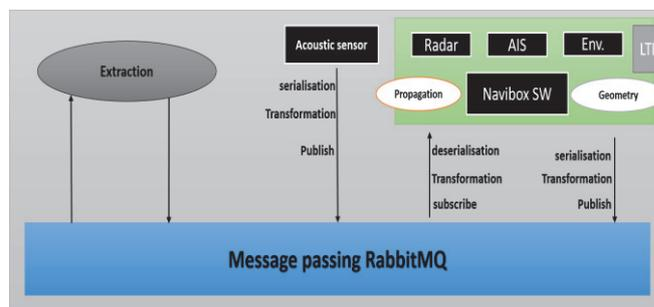
**Figure 3:** SPES integration in the LABSKAUS testbed. Communication is handled with the RabbitMQ message broker
