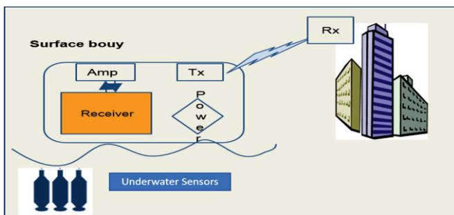
**Figure 5:** Illustration of the Long-term deployed system including a water proof container, underwater sensor components and TX(Transmitter) and RX(receiver).
