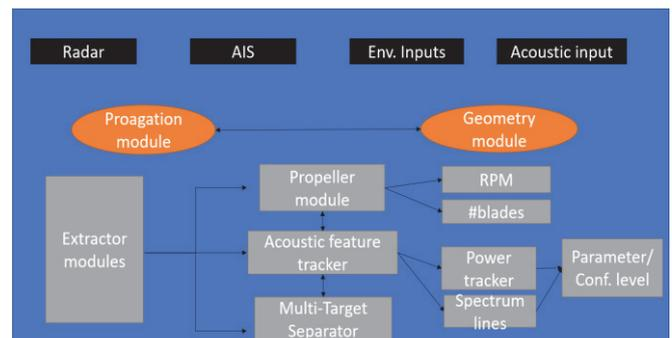
**Figure 2:** The internal modules proposed in the SPES. Three data layers are designed with interchangeability between them.
