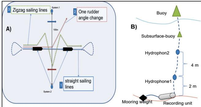
**Figure 4:** Experimental design sketch where A) shows the ship maneuvering plan and B) shows the components of one of the recording systems.
