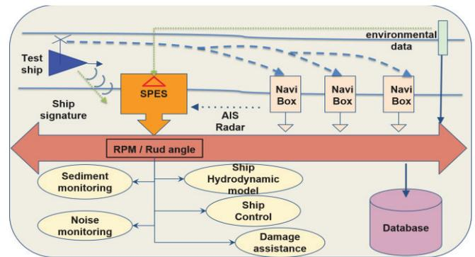
**Figure 1:** Illustration sketch of different components of LABSKAUS reference waterway with proposed integration of SPES.
