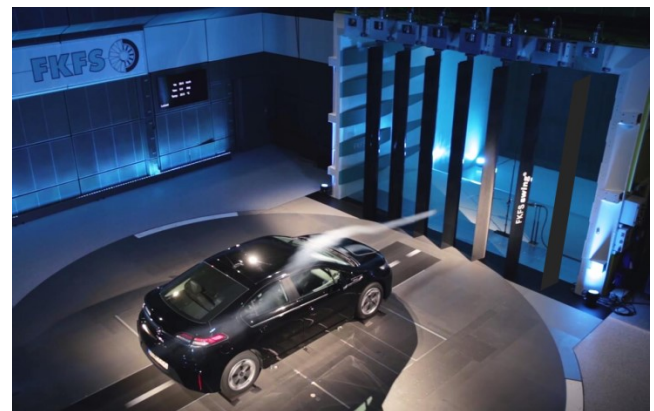
Figure 2: FKFS swing ® in the nozzle exit plane of the full-scale wind tunnel of University of Stuttgart [5]
