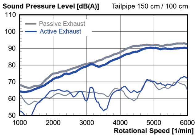
**Figure 2:** Measured overall and 2<sup>nd</sup> EO SPL at the tailpipe of the 4-cylinder gasoline engine at full load (bold lines – OVL; thin lines – 2<sup>nd</sup> EO).
