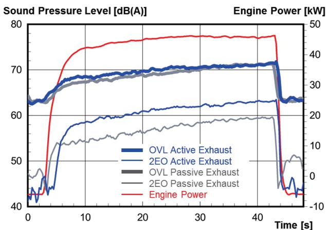
**Figure 3:** Measured overall and 2<sup>nd</sup> EO SPL at the tailpipe of the 4-cylinder gasoline engine and varying load (left axis: bold lines – OVL; thin lines – 2<sup>nd</sup> EO; right axis: red line – engine power at ca. 1.500 rpm).
