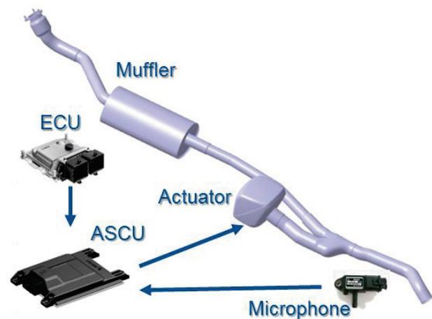
Figure 1: Set-up of an ActiveSilence exhaust system.
