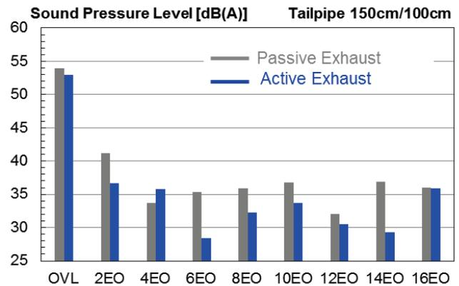
**Figure 4:** Measured SPL at ca. 750 rpm in idle condition at the tailpipe of the 4-cylinder gasoline engine (grey columns – production system; blue columns – ANC system).
