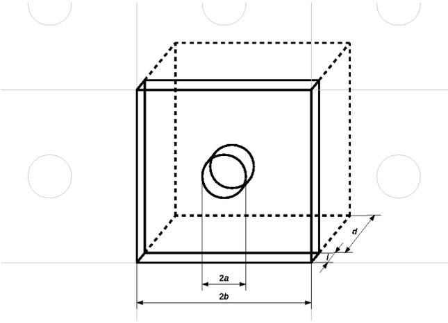
**Figure 1:** Element of a flat perforated liner.
