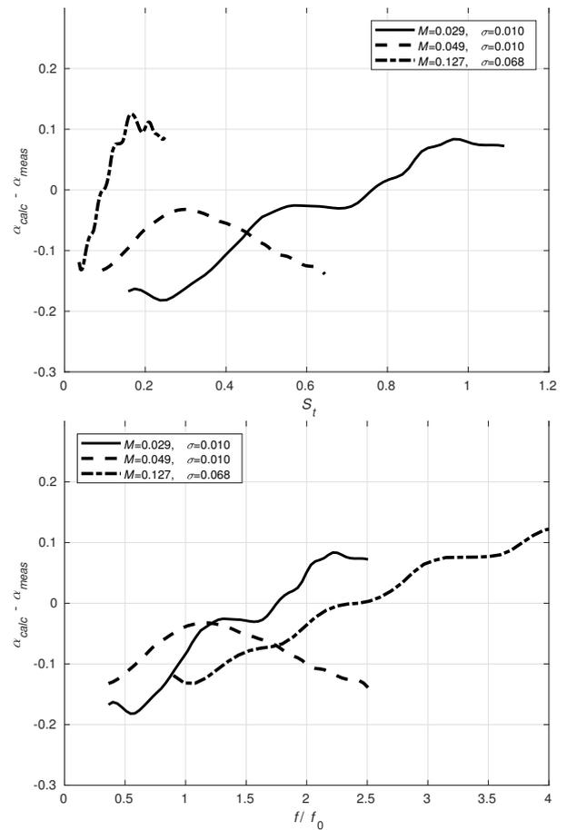
**Figure 4:** Estimated error as a function of Strouhal number (above) and normalized frequency (below) for  $C_c = 0.75$  and  $\delta = \delta_0/2$ .
