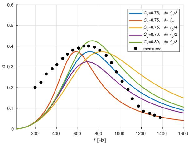
**Figure 3:** The effect of end correction and vena contracta factor on the estimated values of absorption coefficient.
