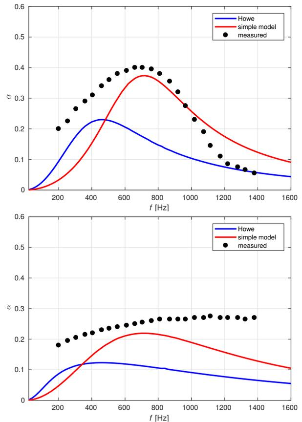
**Figure 2:** Estimated and measured [1] absorption coefficient of a liner in a circular duct: (above)  $M = 0.029$ , (below)  $M = 0.049$ .
