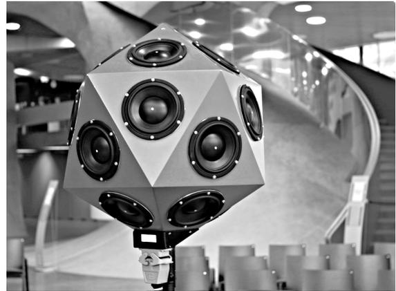
Figure 1: The icosahedral loudspeaker array (IKO)
