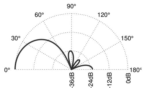
Figure 2: Beam pattern design: 3<sup>rd</sup>-order max- $r_E$  directivity pattern
