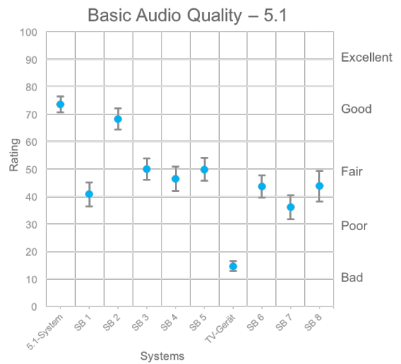
Figure 4: Basic audio quality ratings with 5.1 content, average over all 24 assessors and all samples
