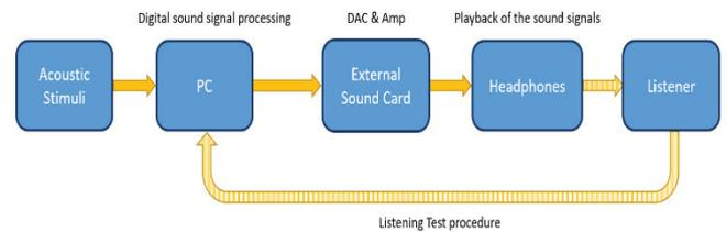
Figure 1: Measurement chain of the listening test
