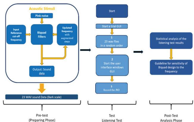
Figure 2: Block diagram of the listening test implementation
