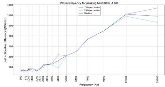
Figure 6: JND for peaking filter gain band -10 dB
