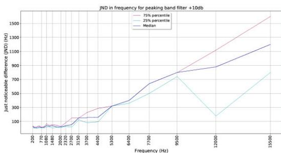
Figure 5: JND for peaking filter gain band +10 dB
