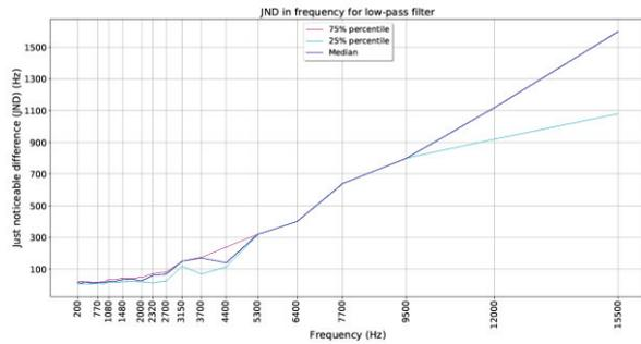
Figure 3: JND for low-pass filter
