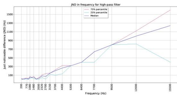
Figure 4: JND for high-pass filter
