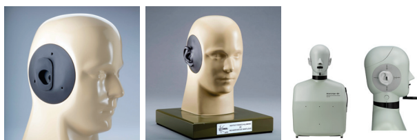
Figure 1: Dummy head configurations: ISL & 3.4, ISL & 3.3, B&K & 3.3 [Taken from [4]](from left to right).
