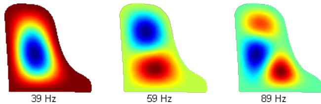
Figure 11: Solid plate modes in case of hypothetical material valid in deterministic and stochastic case as well (Standard deviation is approaching for 0%).
