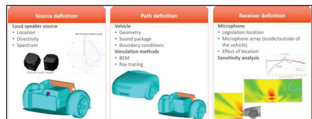
Figure 2: Illustration of the source/path/receiver proposed to simulate the pedestrian safety problem.
