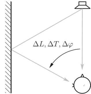
**Figure 1:** Illustration of a typical setup used to study the echo threshold. Compared to the direct sound, the specular reflection arriving at the listener's ears is attenuated by  $\Delta L$ , delayed by  $\Delta T$ , and spatially separated by  $\Delta\varphi$ .
