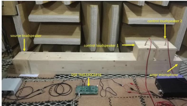
Figure 3 – The experimental arrangement of duct ANC system in the anechoic room.
